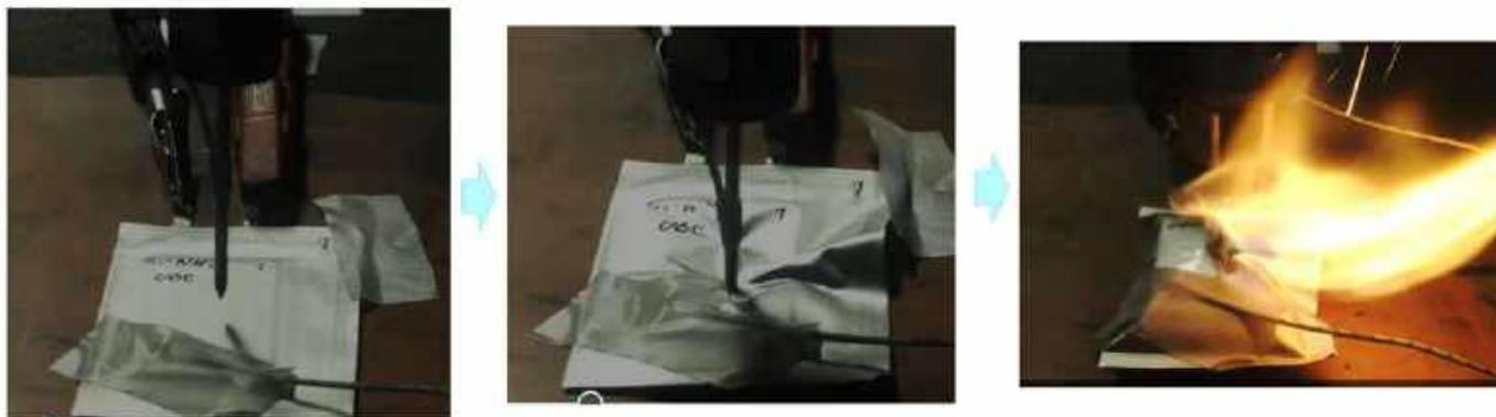
Figure 30: Chronological sequence: cell before nail penetrates (left), nail penetrated the cell (middle), thermal runaway (right).
