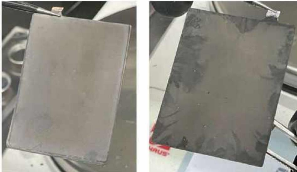
**Figure 17: Visual assessment of the BL-1Ah anode (left) and cathode (right).**
