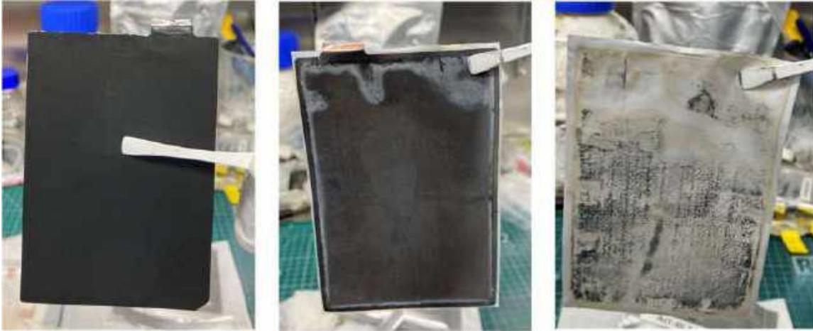
**Figure 16: BL-5Ah pouch cell post-mortem components including cathode (left), anode (middle) and separator sheet (right).**
