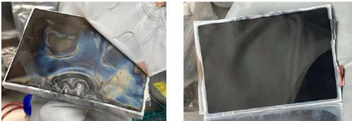
Figure 24: Damaged anode sheet with 'swollen' active material sections in wave-shape (left) and cathodes in good condition without any abnormalities (right).
