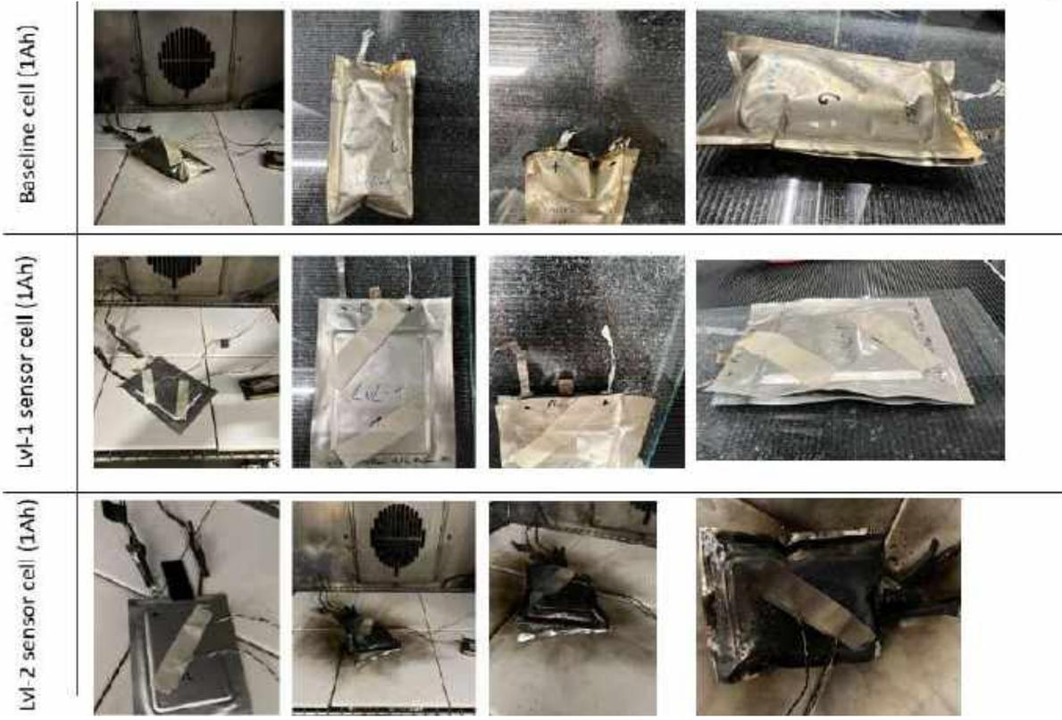
Figure 31: 1 Ah baseline, Level-1, and Level-2 sensor cells during and at the end of the heating test
