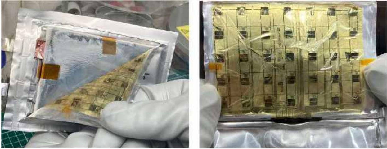
Figure 22: Opened L1-5Ah pouch cell with direct vie on the integrated L1 sensor unit.
