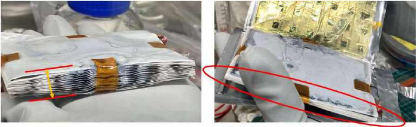
Figure 23: Cell stack thickness comparison. 'Swollen' stack side where sealing area was located (left) vs. opposite stack edge (right).
