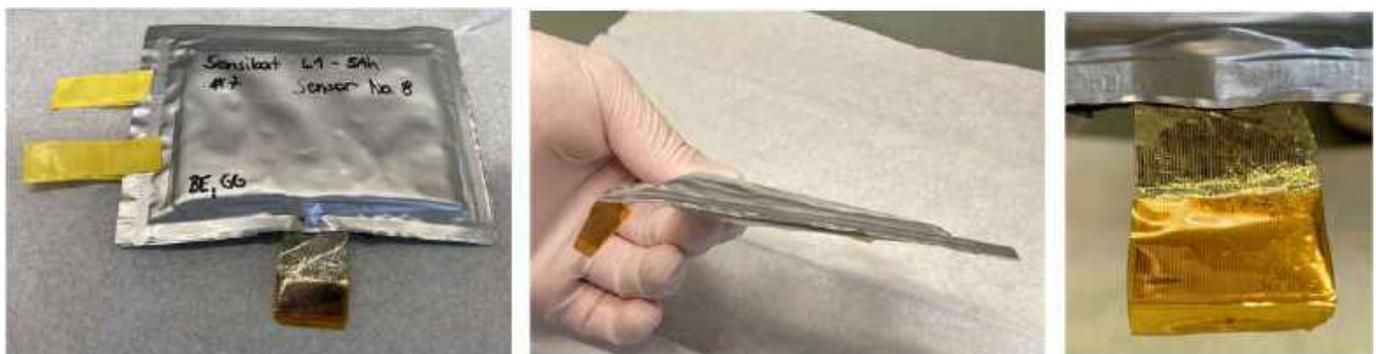
Figure 21: Swollen L1-5Ah pouch cell with visible sensor trace damage.
