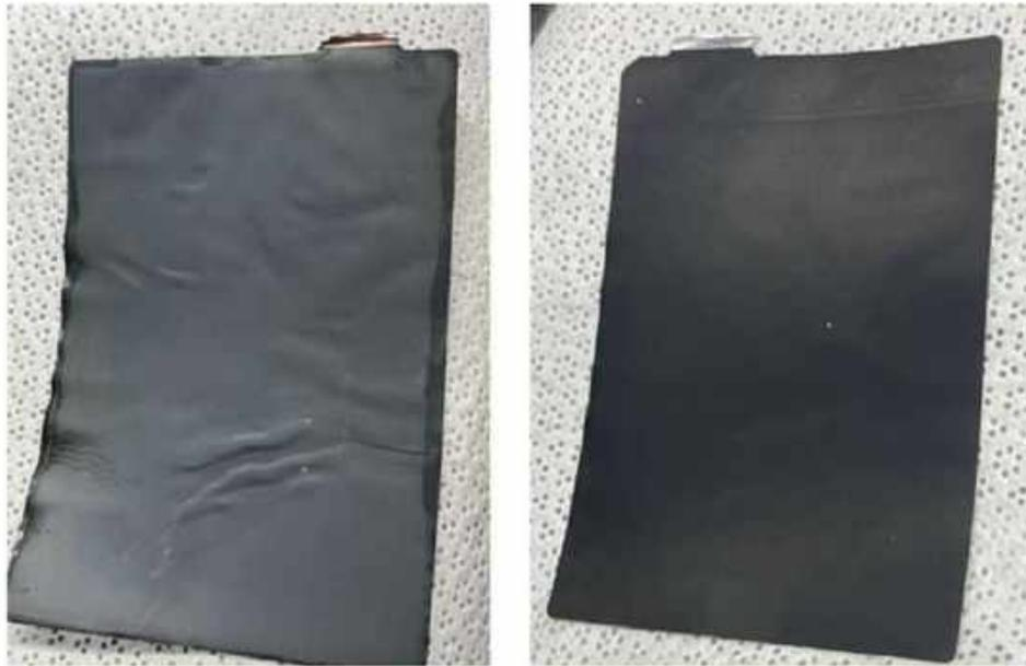
Figure 20: Visual assessment of the L1-5Ah anode (left) and cathode (right).
