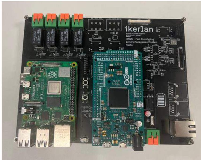
Figure 23: BMS Master prototype
