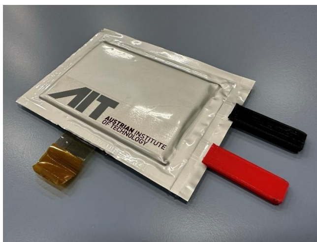
Figure 1: SENSIBAT Final L1 5Ah pouch cell with integrated sensor unit
