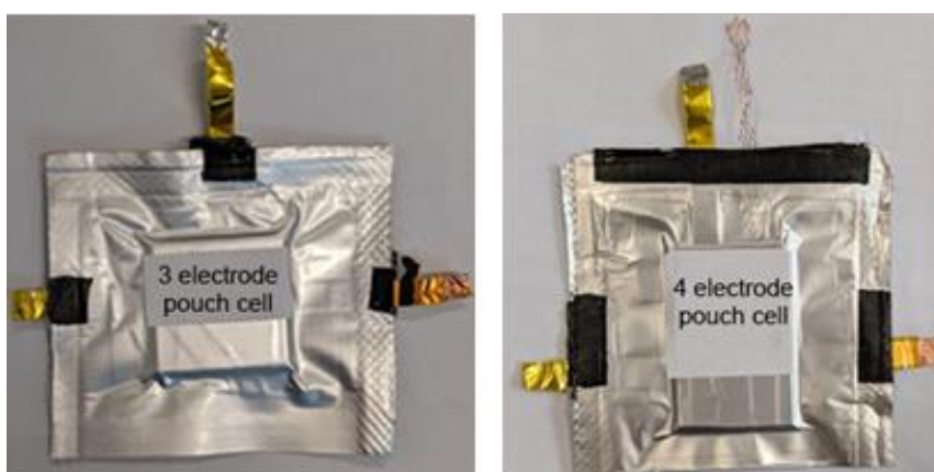
Figure 3. Pouch cells in three and four-electrode configurations, as resulting by the incorporation of sensing electrodes printed on Celgard 2500 separators.
