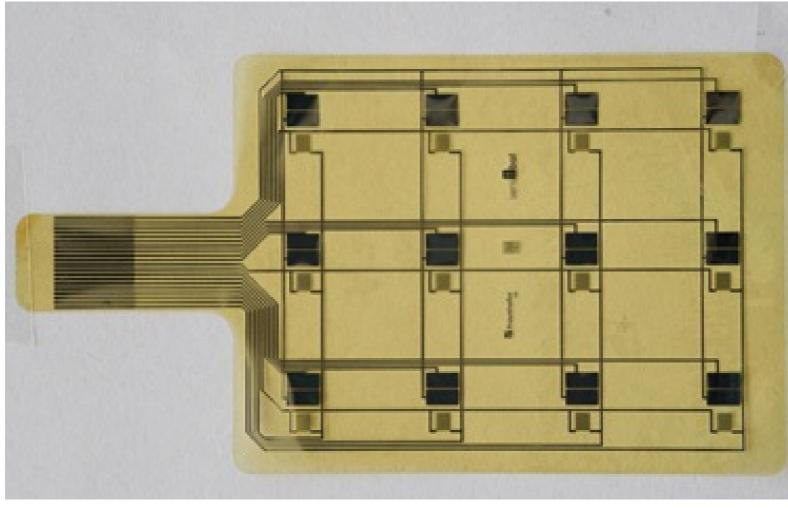
addressing as well as 12 capacitive pressure sensors in common rail configuration.
