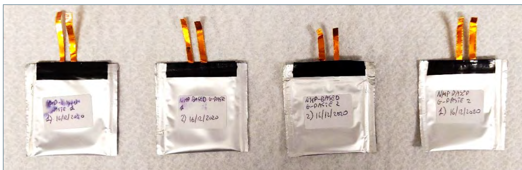
Figure 10. Four complete bags with embedded electrodes. Sample 3-1-1, Sample 3 1-2, Sample 3-2-1, Sample 3-2-2.
