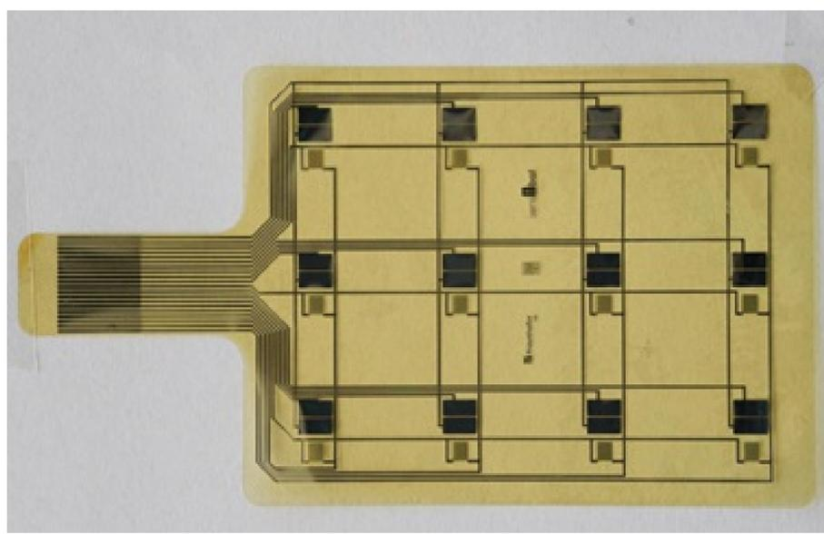
In the figure above you can see the SENSIBAT Level 1 sensor matrix designed for 1 Ah battery cells before encapsulation. The matrix holds 12 resistive temperature sensors for cross-point array addressing as well as 12 capacitive pressure sensors in common rail configuration.
