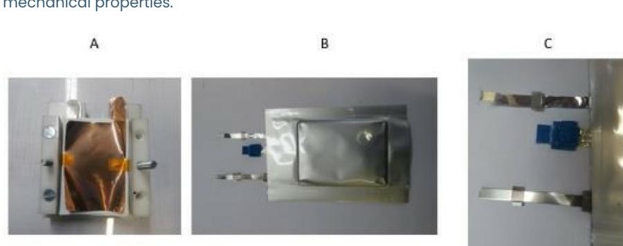
In the figure above you can see the electrode stack during construction at VARTA (A), Finished cell with embedded sensor dummy (B), feedthrough area (C).
