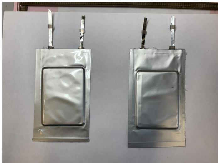
Figure 6. SENSIBAT 1Ah baseline pouch cells produced at VAR
