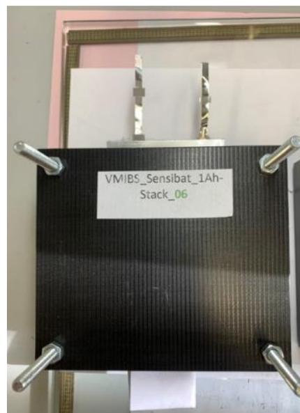
Figure 7. SENSIBAT 1Ah baseline pouch cell produced at VAR with applied jig
