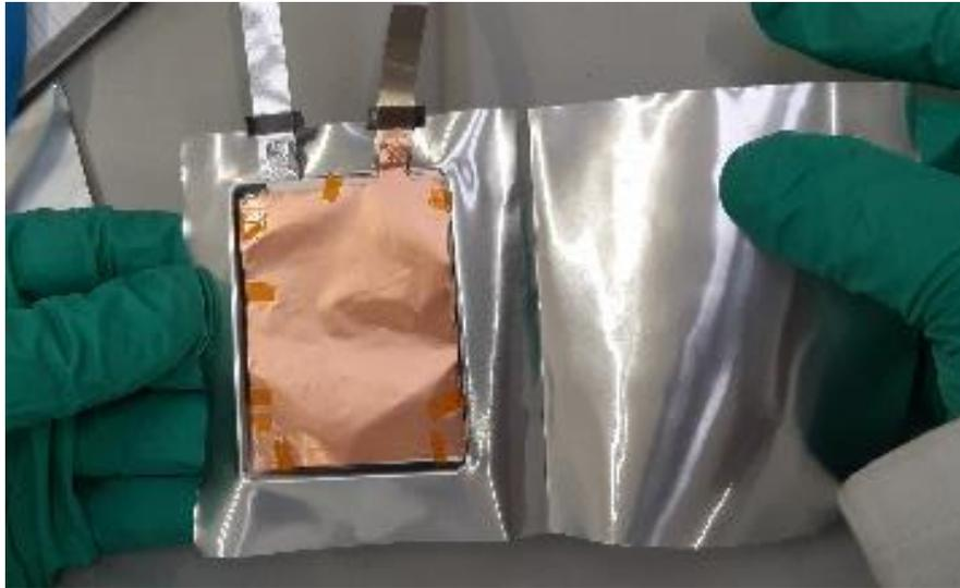
Figure 8. SENSIBAT 1Ah baseline pouch cells produced at ABEE
