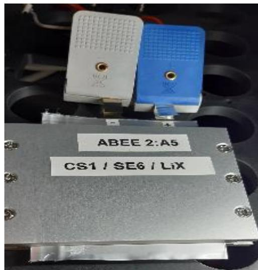
Figure 9. SENSIBAT 1Ah baseline pouch cell produced at ABEE with applied jig
